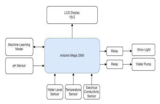
Fig 1. Embedded System Block Diagram
